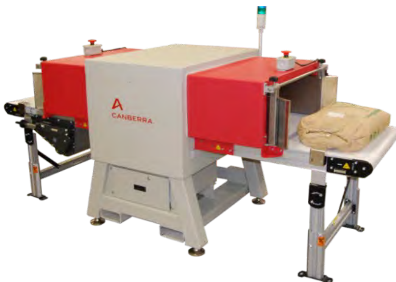
Figure 9: Automatic Rice Bag Counter.
