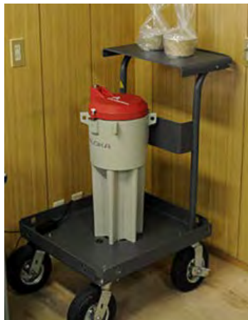
Figure 5: Transportable NaI food assay system.
