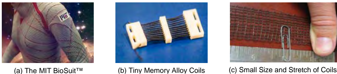
Figure 6: The heat shrink MIT BioSuit™ and the tiny stretch memory coils.
