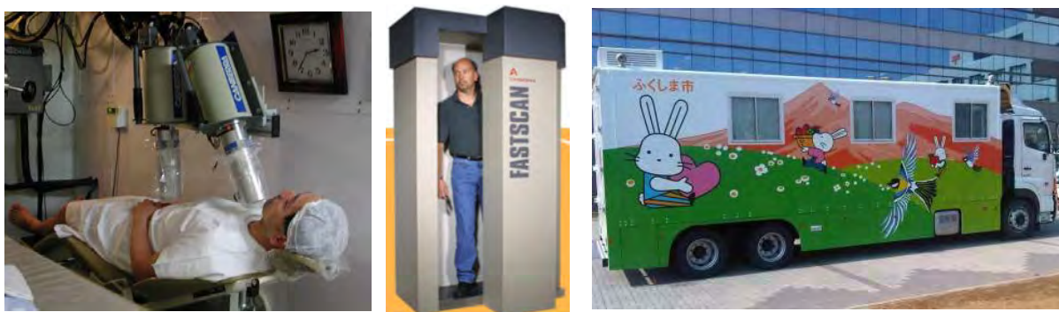
Figure 6: Various WBC systems: left is the JAEA-Tokai facility; middle is the Canberra FastScan; right is one of the trucks containing a FastScan.
