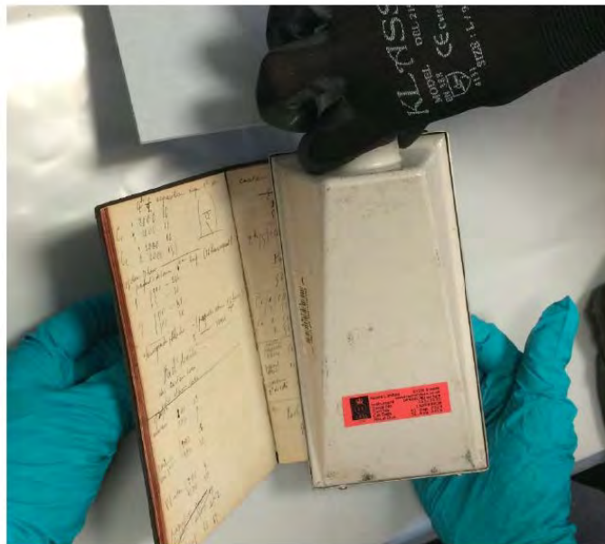
Figure 3: Direct monitoring of the Marie Curie notebook using DP6 probe
