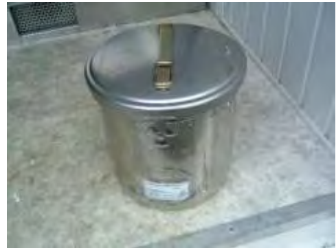
Figure 3: B(U) package for Am-241 sources
