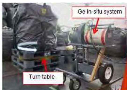
Figure 3: The measurement of SS with Ge in- situ system.
