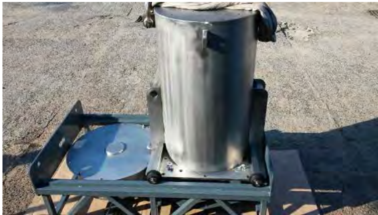
Figure 2: Newly manufactured transfer Cask showing position of the borehole. Photo courtesy of Mr Janos Balla.
